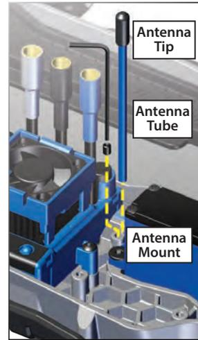
**!** To prevent loss of radio range do not kink or cut the black wire, do not bend or cut the metal tip, and do not bend or cut the white wire at the end of the metal tip.
