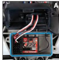
**Note:** For best performance, it is recommended that the receiver be installed in the original orientation as shown.
