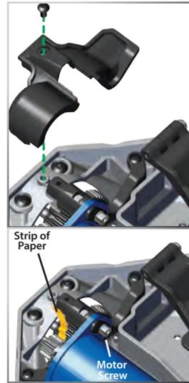
If you choose to do so, you can also set the gear mesh manually without using the fixed gear adapter. With the adapter removed, loosen the motor screw. Cut a narrow strip of notebook paper and run it into the gear mesh. Slide the motor and pinion gear into the spur gear. Retighten the motor screw, and then remove the strip of paper. You should be able to run a fresh strip of paper through the gears without binding them.
